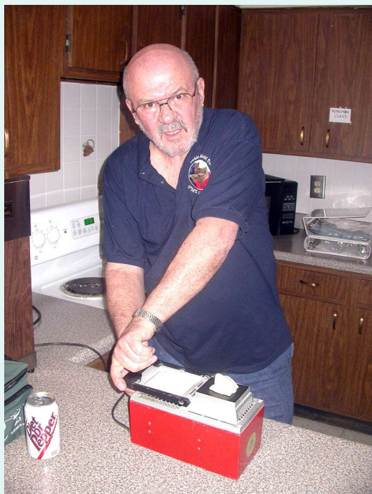
John Estes using his trusty old vac-u-form machine to make a canopy for Fabian Nevarez.
